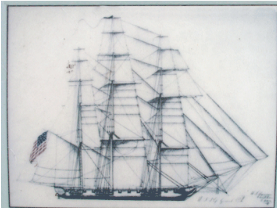
This spar and sail plan for the General Pike was drawn by Charles Ware and shows the vessel's appearance when completed after the battle. Courtesy of the National Archives.
